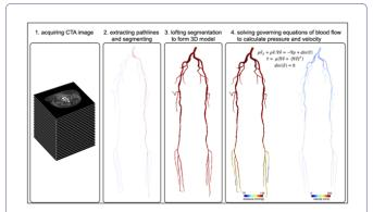
**Figure 1:** Image-based modeling procedure. A vascular model is constructed by segmenting the peripheral arteries from a computed tomographic angiography image volume. Computational fluid dynamics are used to compute flow and pressure throughout the model.
